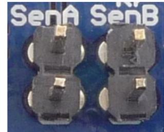
Fig.3 - Current sensing jumpers
