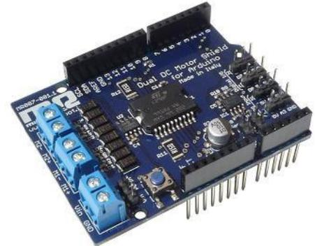
The *Dual DC Motor Shield* is a shield that has been projected to enable an Arduino board to drive two brushed DC motors or one 4-wire two-phase stepper motor, controlling the speed and direction of each one independently.
